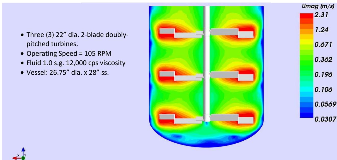
Figure 1. Velocity Contours Plot with a ProQuip Doubly Pitched Axial impeller.
