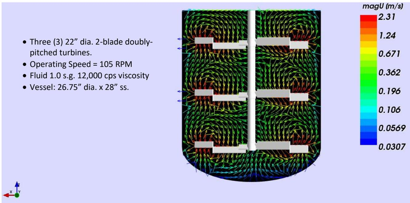
Figure 2. Velocity Vectors Plot with a ProQuip Doubly Pitched Axial impeller.
